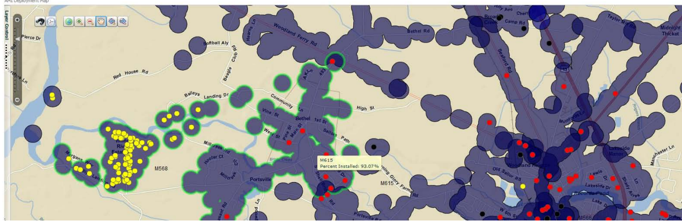
An example dashboard shows the percent saturation of meter reading routes by AMI meters installed vs. planned locations to be installed. A subset of the AMI meters is colored by AMI status values.
