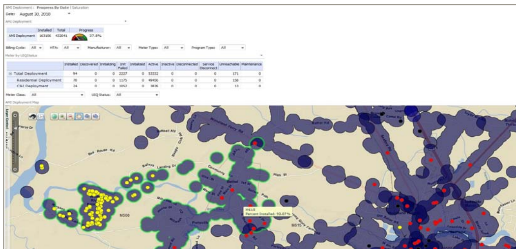
An example dashboard shows the percent saturation of meter reading routes by AMI meters installed vs. planned locations to be installed. A subset of the AMI meters is colored by AMI status values.
